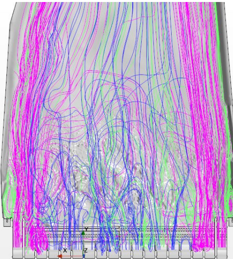
Figure 24 – Streamlines for 125 Kcfs Spill and 25 foot Tailwater
